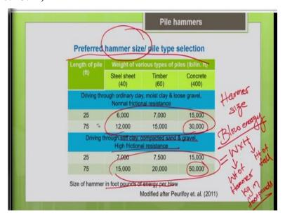
So, makes this about the how to select the pile hammer based upon your weight of your pile, length of your pile and the material type. So, hammer size, here we are going to select the hammer size, so hammer size is generally defined in terms of blow energy, hammer size is defined in terms of blow energy, so how do you determine the blow energy? It is nothing but W into H, W is your weight of hammer and H is your height of fall, so kg meter or whatever.
