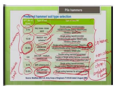
Now how to make the pile hammer selection with respect to your soil type, as I told you we can classify the soil into different categories. So, based upon there are some standard tests to categorize the soil into different categories. Like once this test is your standard penetration test where you find what is the number of blows needed for the standard penetration. So, based upon the number of blows you classify the soils into different categories are shown here.
