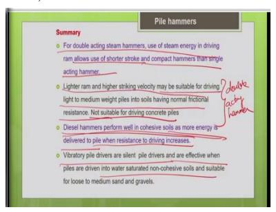
For double acting hammer, use of steam energy in driving ram allows use of shorter stroke and compact hammers than the single acting hammer. So, double acting hammers are basically smaller in size and they go with shorter stroke when compared to single acting hammer. So, they have basically recommended for the soil with normal friction resistance and for light to medium weight piles.
