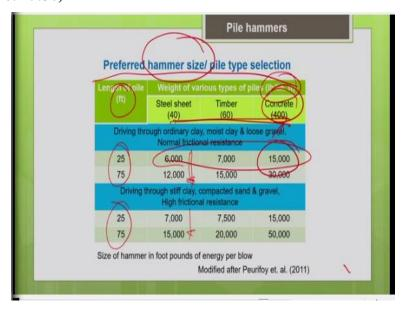
As your length of pile increases you can see that the blow energy requirement increases this is your pile length is given in feet. And another important thing to be noted is as your weight of pile increases, here they have given the weight per unit length that is pounds per linear feet. As your weight of the pile increases you can see that your blow energy requirement also increases.
